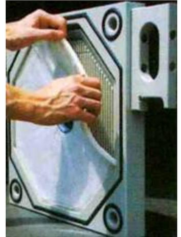
Caulked And Gasketed Biodiesel Filter Plates
